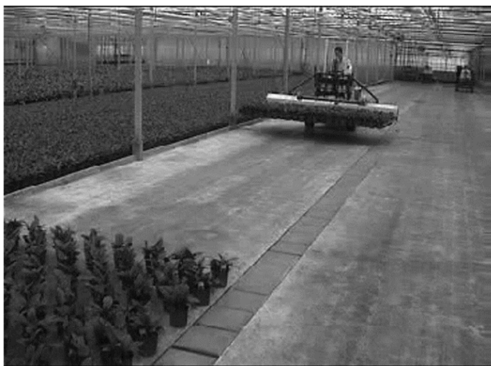
Figure 1. A typical fork system being used to move plants in a nursery.
